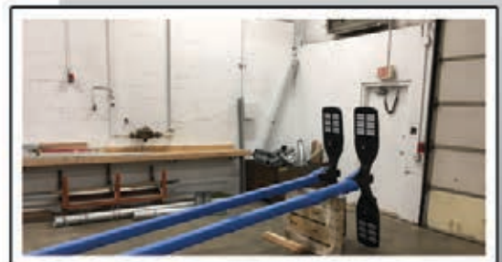
Pre-Assembled Light Poles
