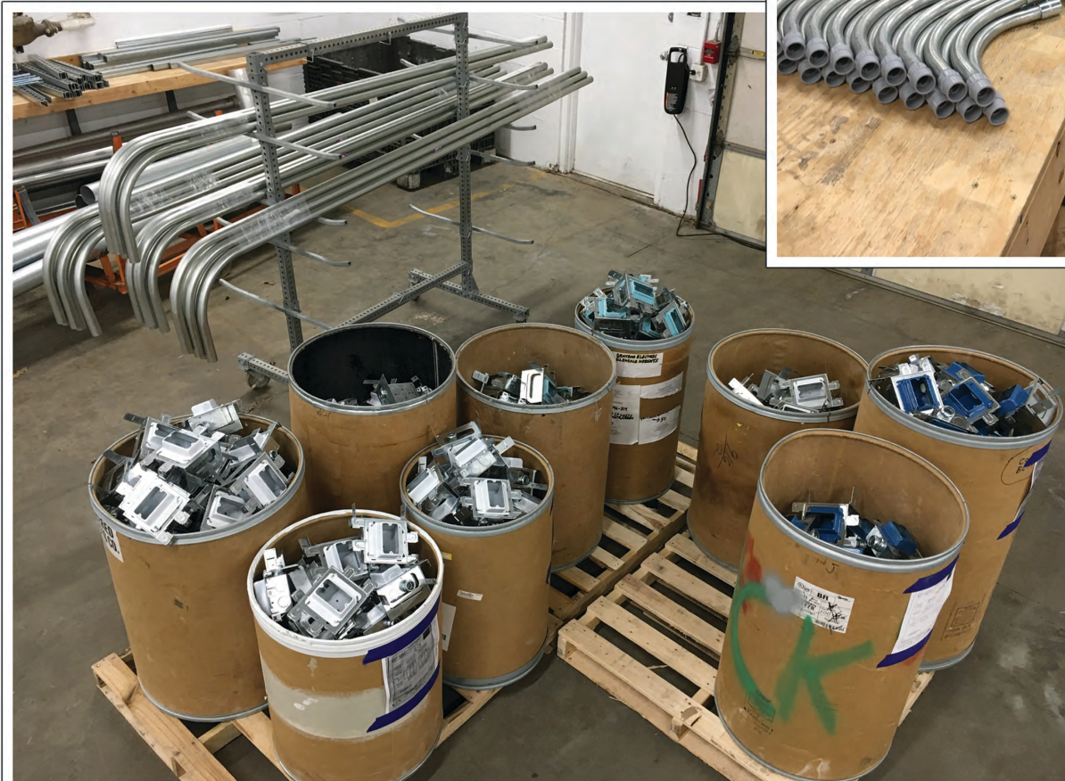
Right Side of Picture: 1900 Boxes with Drywall Ring, and Stud Bracket. Uses: Lighting, power, and data in-wall rough-in.
